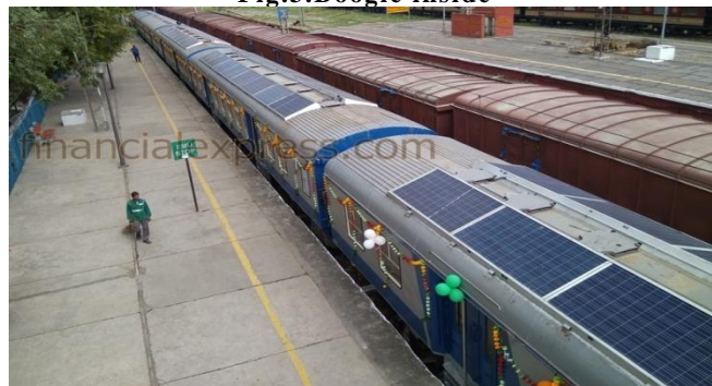
Fig.4Top view of PV panel
