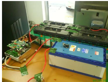
Fig 9: Implementation of HESS (EMU is left, central is LiFePO 4 LIB pack and right is UC pack)
