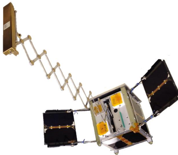
Fig. 1: Photograph of KSAT2, developed by a consortium with Kagoshima University. A main body at the bottom is a 10-cm cube. The outers are solar cell panels (both sides) and a pantograph (top) for stabilization.
