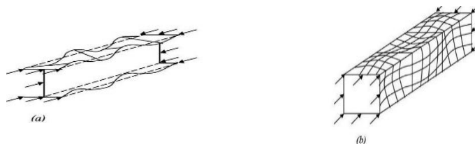
Fig. 2- Local buckling of (a) open section, (b) closed sections [6][6]
