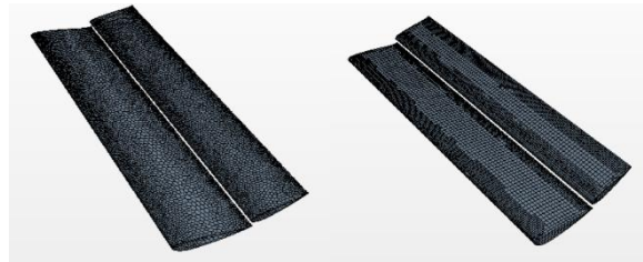
Fig 4: : Mesh of a wing model using polyhedral (left) and trimmer (right) mesh model.
