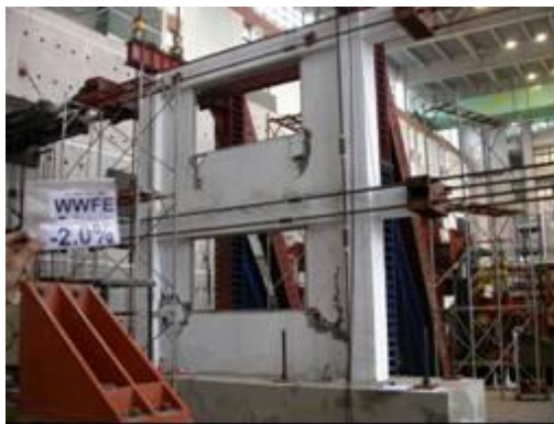
Photo 5. Cracking happened at the corner of the walls
