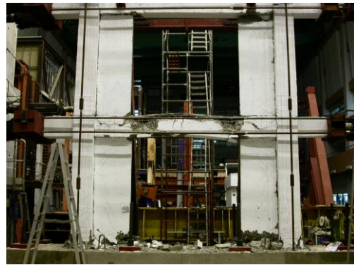
Photo 2. The final failure on specimen FER
