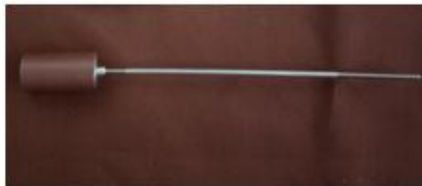
c. Piston and piston rod assembly
