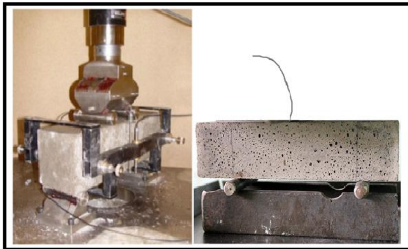
Fig 3 - The equipment of pull-out Figure 5 pull-out specimen after cutting sample preparation.
