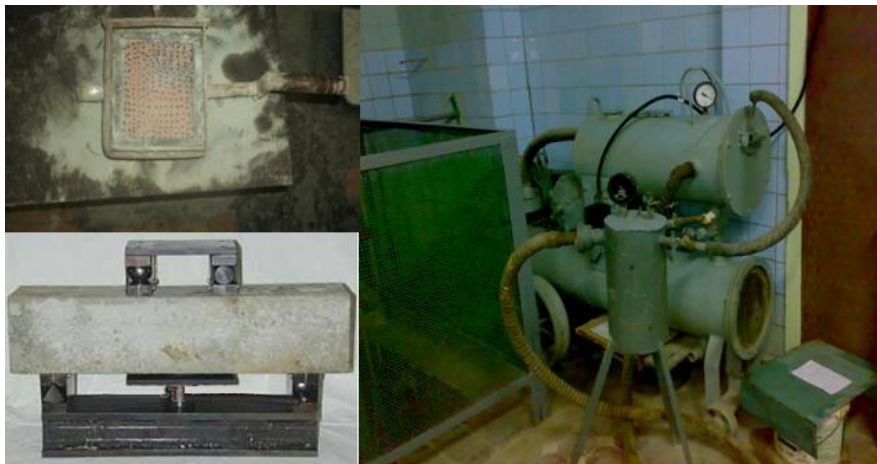
Fig 1 - Laboratory equipment for sample preparation by method vibr-vacuumizing.
