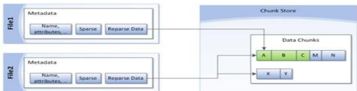
Fig 5. On-disk transformation of files during data deduplication
