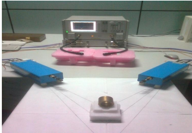
Fig. 8: Cold test set up of high frequency gyrotron cavity [8]
