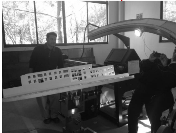
Fig 8. New heliodon's performance evaluation on site for an architectural model.
