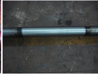
Fig.13. Shaft ready for reuse
