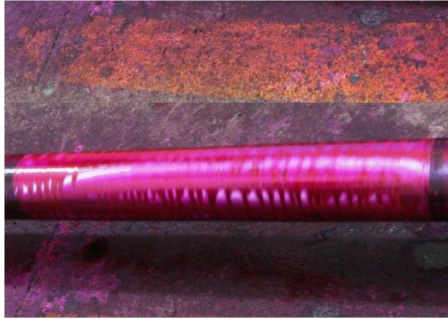
Fig.12. DP testing of welded shaft
