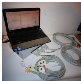
Fig. 8 Device for reading epithelial potential differences in breast 10-lead cables
