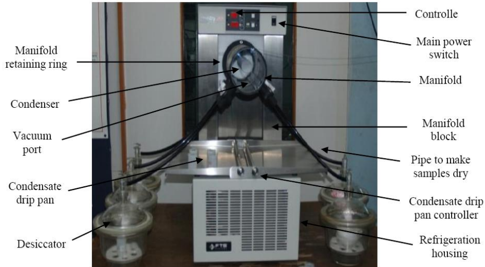
Figure 5: Photograph of the micro-processor controlled Freeze Drier.
