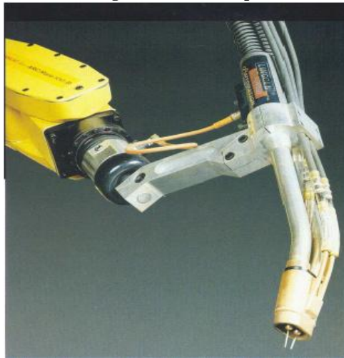
Fig 6. Torch for tandem welding produced by Lincoln Electric. [2]
