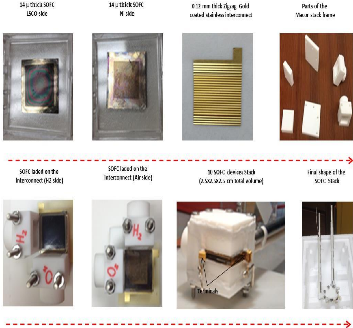
Fig 3. Thin solid oxide fuel cells stacking process
