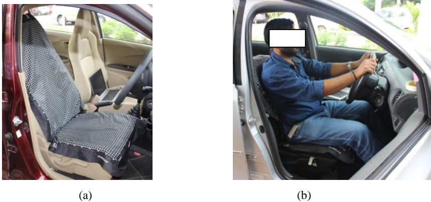
Fig 5. (a) Pressure mapping set-up (b) Pressure mapping process
