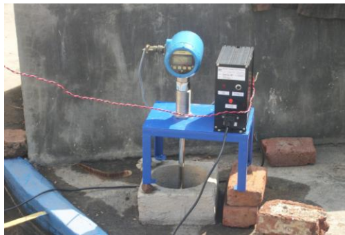
Fig. 7: GWR Type Sensor Used In Transient Type Water Level Model
