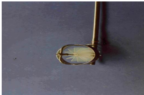
Fig. 8: 50mm Diameter Propeller Type Current Meter Used For U > 100 cm/Sec
