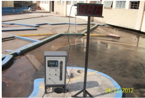
Fig. 6: WSF Type Sensor Used In Steady Type Water Level Model
