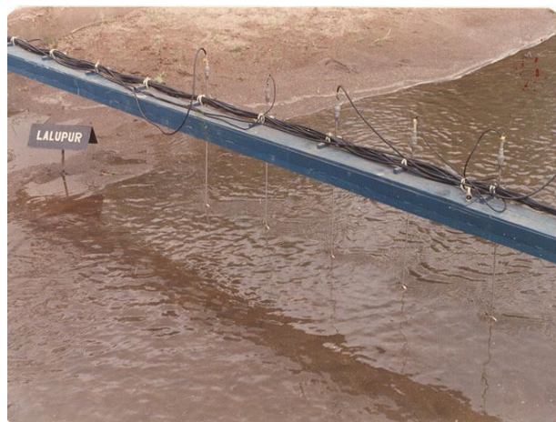
Fig. 5: Measurements of Water Velocity and Discharge on River Model.
