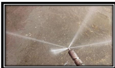
FIG -20. 4 HOLE NOZZLE Z TYPE RETROFIT WITH HOLES
