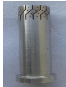
FIG-4. MODEL OF THE Z TYPE CUT WITH HOLES RETROFIT-14 PROJECTIONS
