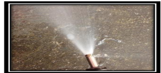
FIG -19. 4 HOLE NOZZLE Z TYPE RETROFIT WITHOUT HOLES
