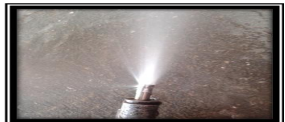
FIG -21. 4 HOLE NOZZLE STRAIGHT TYPE RETROFIT WITH HOLES
