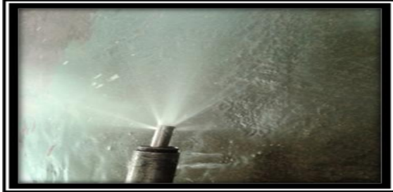
FIG -24. 5 HOLE NOZZEL STRAIGHT RETROFIT WITHOUT HOLES
