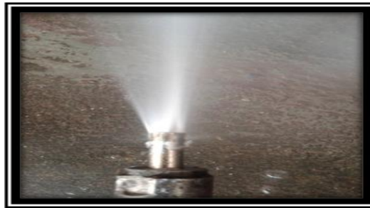
FIG -26. 5 HOLE NOZZLE Z TYPE RETROFIT WITH HOLES
