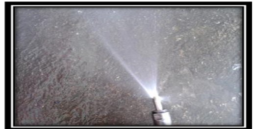
FIG -21. 4 HOLE NOZZLE STRAIGHT TYPE RETROFIT WITH HOLES
