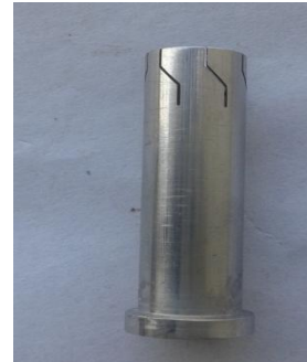
FIG-3. MODEL OF THE Z TYPE CUT RETROFIT-7 PROJECTIONS
