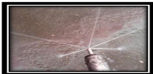
FIG -20. 4 HOLE NOZZLE Z TYPE RETROFIT WITH HOLES
