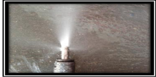
FIG -25. 5 HOLE NOZZLE STRAIGHT RETROFIT WITH HOLES
