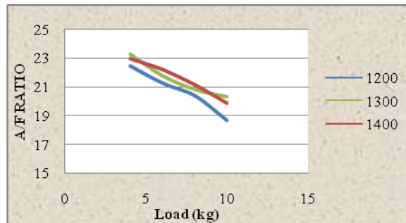
Fig.4 Air-Fuel ratio on Diesel mode
