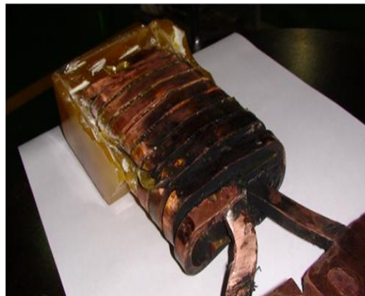
Fig. 11 Deformation of helical-type forming coil
