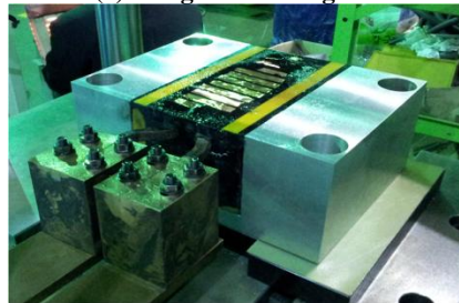
(b) Manufacturing the forming coil Fig. 7 helical-type forming coil
