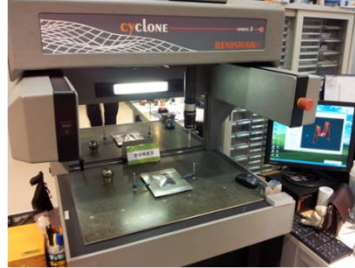
Fig. 15 3D scanning for measuring the deformation depth
