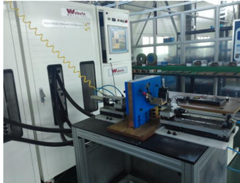
Fig. 2 Magnetic pulse welding system for this study
