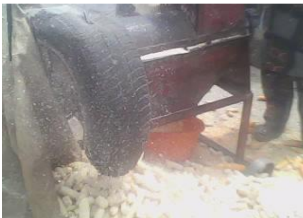
Plate 3a: Cobs Outlet Covered with Tyre to Prevent Flying Over
