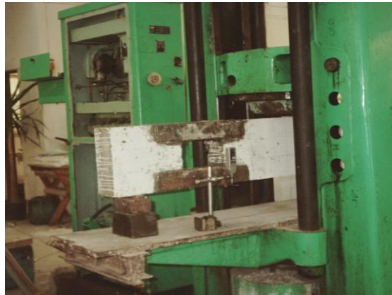
Fig 6: the setup of beam test
