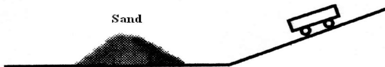
Fig.3. Cart going down for a sloping plane and being less and less rubbing in his way for the horizontal plane
