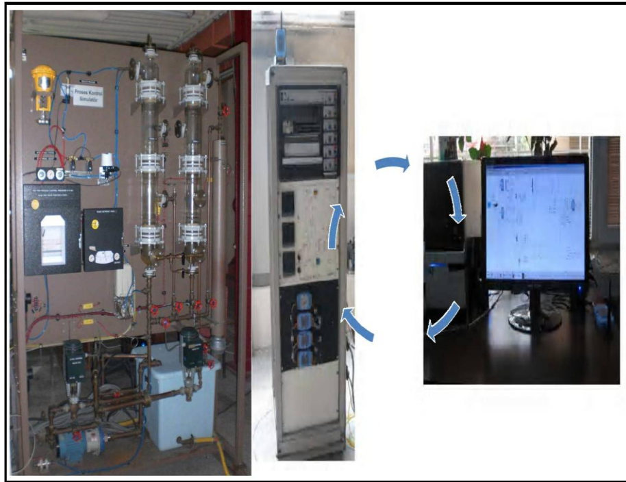
Fig. 1 Experimental system: Process simulator, control panel and computer on-line connected to the process simulator with wireless technology
