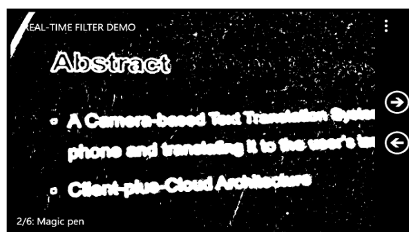
Fig.8 Applying Threshold Filter (which is a Combination of Grayscale and Contrast Filter)
