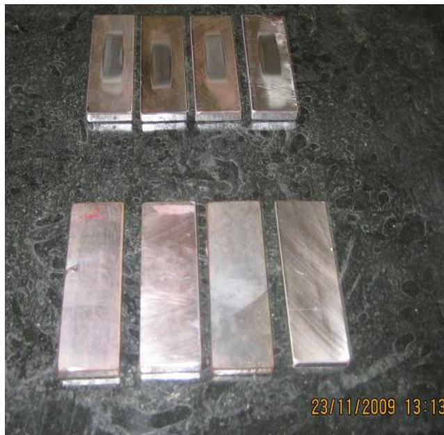
Fig 1: Standard test specimen (75x26x6 mm)
