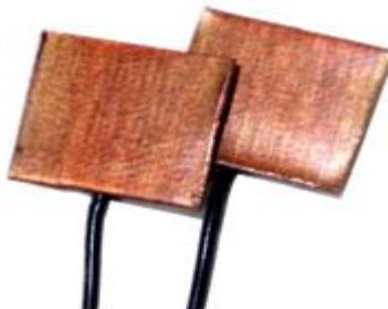
Fig 8: Copper plates used to measure GSRs
