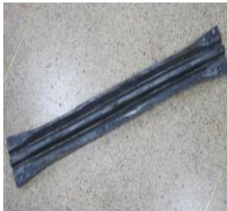
Fig. 11 Morphology of door beam after hot stamping
