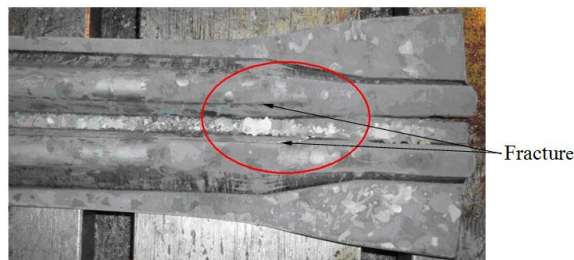
Fig. 9 Door beam with fracture in actual production
