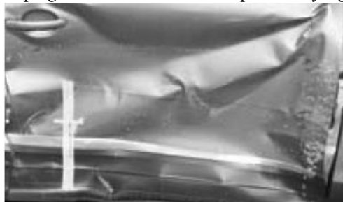
Fig 15. Automobile door after side impact test
