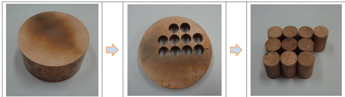
(a) oxygen-free copper(C10100) (b) Cutting by a wire-electric spark machine (c) Specimens Fig. 2 Specimens of the compression test for oxygen free copper
