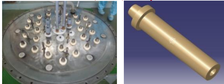
Fig.1 Ingot furnace and electrode body part of solar light
