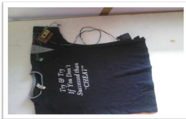
Fig.4 Wearable TShirt with sensors fit
