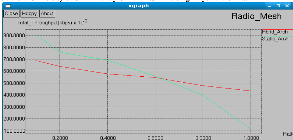
Fig IV: Presents the hybrid architecture compared with the static architecture. In this throughput of hybrid architecture is higher than the static architecture. Here x axis denotes the ratio skewed and y axis denotes the throughput. Green colour curve denotes static architecture results and red color curve denotes hybrid architecture results.
