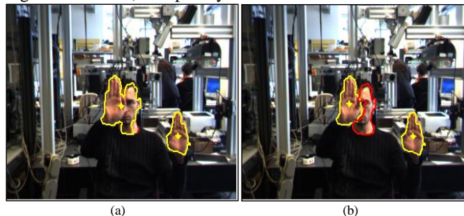
Fig. 3. Solving overlapping problem between hand and face using depth map. (a) 2D image in which the face and the left hand are occluded. (b) 2D image with labeled hands and face without occlusion.
