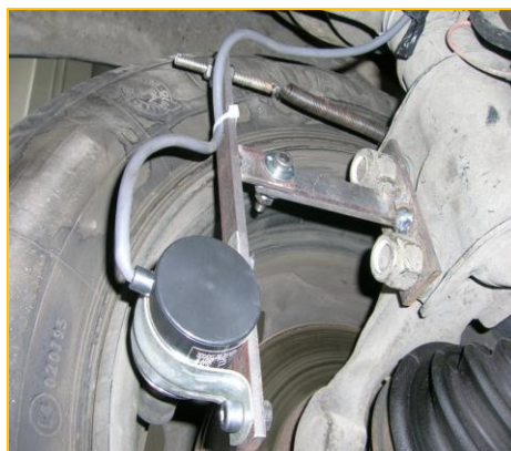
Fig 3. Encoder fitted to the vehicle wheel
