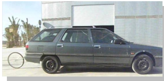
Fig 4. Fifth wheel, or drive wheel.
