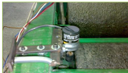
Fig 2. Encoder fitted to brake roller tester
