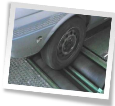
Fig 1. Test 1 measuring on the brake roller tester at the MOT centre.
