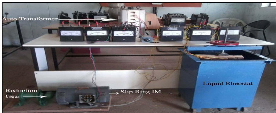
Fig1. Experimental Setup for Conventional speed control Method
