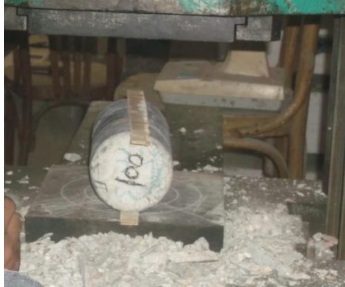
Fig 6. Setup of the splitting tensile test.
