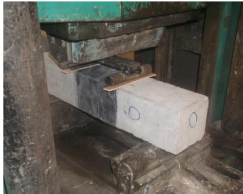
Fig 7. Setup of the flexural test
