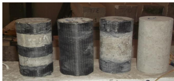
Fig 2. Different forms of CFRP wrapped around cylinders
