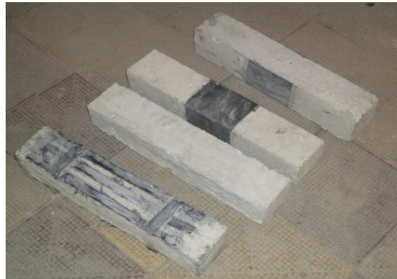
Fig 3. Different forms of CFRP wrapping on prisms
