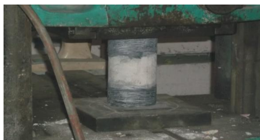
Fig 5. Setup of the compressive test
