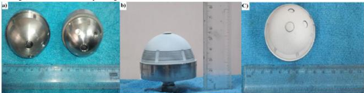
Fig 10. (a) Uncoated Acetabular Cup (b) & (c) High quality HAp Coated Acetabular Cup (front & top view respectively) [HAp powder of particle size 75-112 micron supplied by IFGL Bioceramics Ltd] [16]
