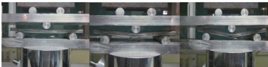
Fig 8. Three point bending strength test Configuration [16]
