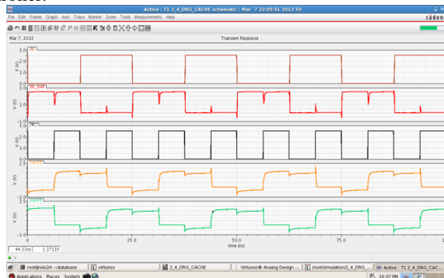
Fig. 7. Waveforms of drowsy memory circuit
