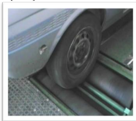
Fig.2: Test 1 measuring brake force on the brake roller tester at the MOT station.
