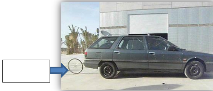
Fig.3. Encoder on Fifth wheel, Test 2
