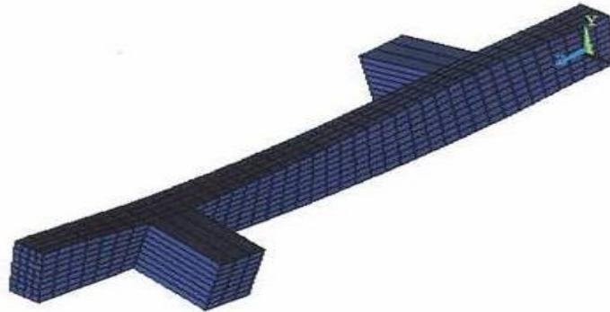
Fig 9. Deformed shapes of beam B1
