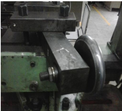
Fig 3a.spinning lathe with single roller
