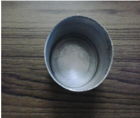
Fig 4b. Tube formed Cup (Top-view)
