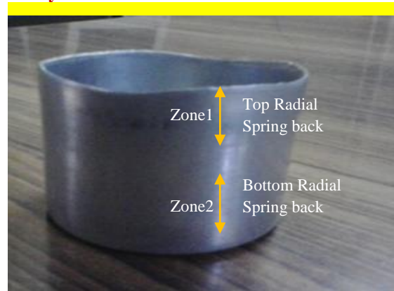
Fig 4c. Tube formed Cup Radial Spring back measurement zones
