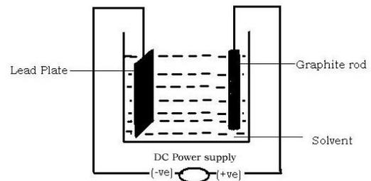
**Fig 1: Line diagram of electrode position**
