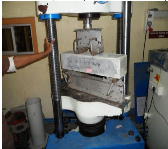
Fig 6: set up of Universal Testing Machine for flexural strength
