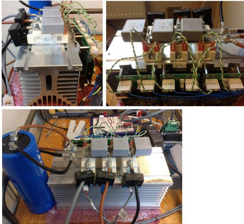
Fig. 7. The Top Pictures Presents The Drive Circuit Connected To The IGBT On The Heat-Sink, Whereas The Lower Picture Shows The Installed Hall-Sensors, Implemented To Measure The Flowing Current.
