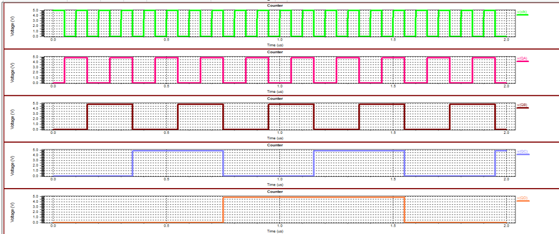
Fig 15 simulation result of four bit reversible asynchronous bidirectional counter
