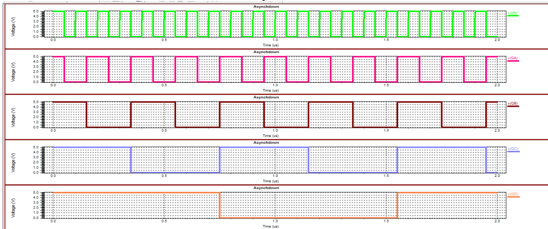
Fig 14 simulation result of four bit reversible asynchronous down counter
