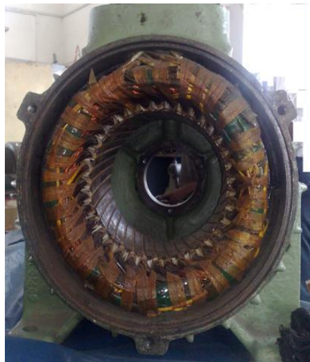
Fig 6. Experimental Stator of PMSRM
