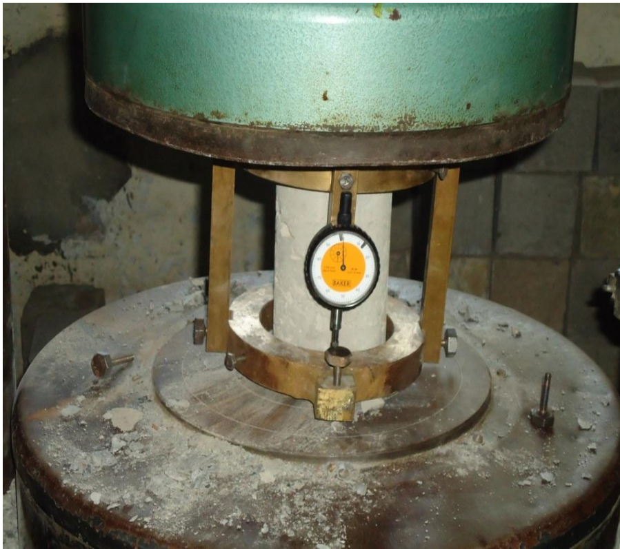
Fig 1: Setup of Modulus of Elasticity
