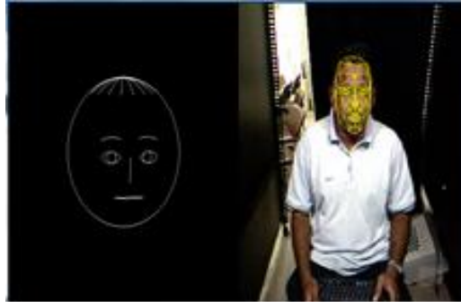
Fig.12 Visualizing User Expression Using RGB-D Camera
