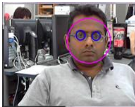
Fig. 10 Detection Result for Face and Eyes ROI
