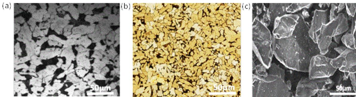
**Fig.2. Microstructures of: (a) AISI 1018, (b) API X42 and (c) aluminum oxide particle size distribution.**
