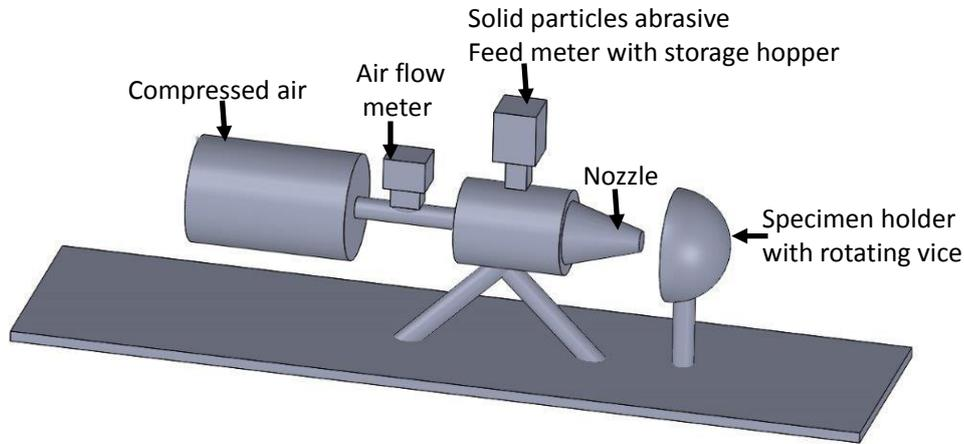
**Fig.1. Schematic diagram of the sand blaster erosion machine**
