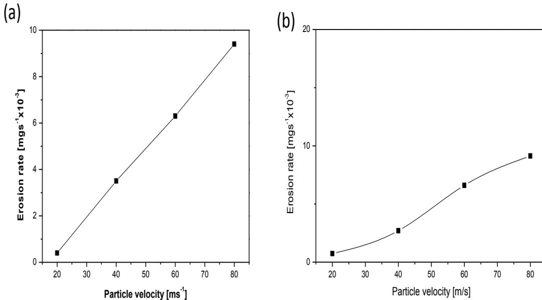
Fig.3. Erosion rate Versus Particle velocity for: (a) API X42 and (b) AISI 1018 steel materials
